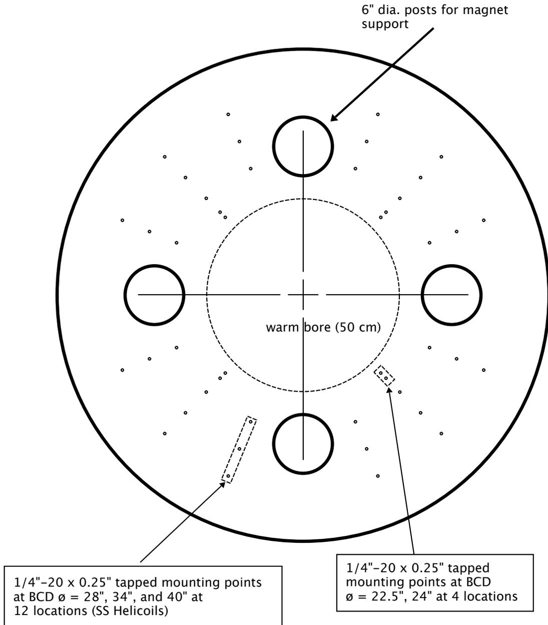
Drawing: MDPX - Cryostat mounting points
