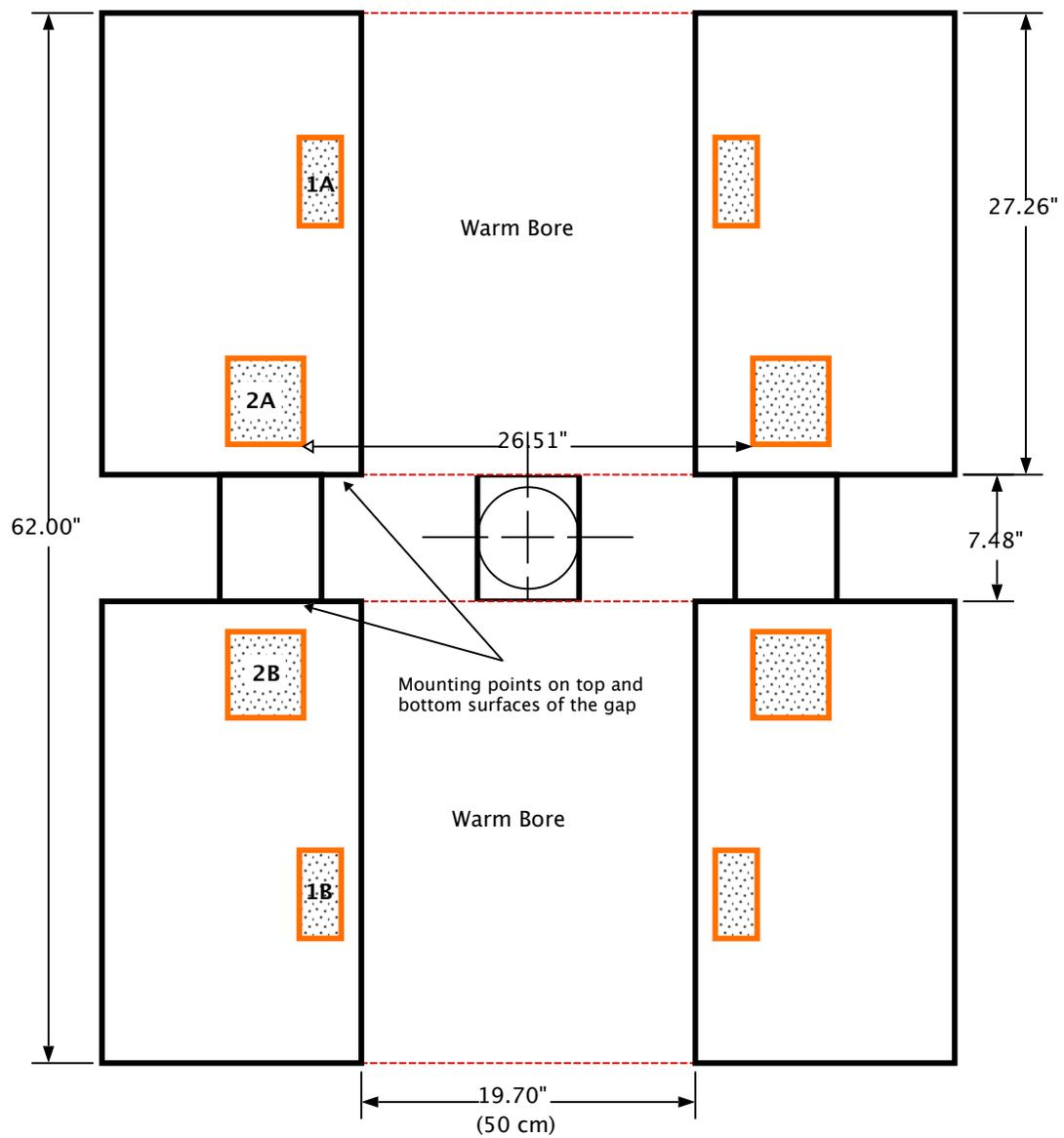
Drawing: MDPX - Magnet Cryostat
