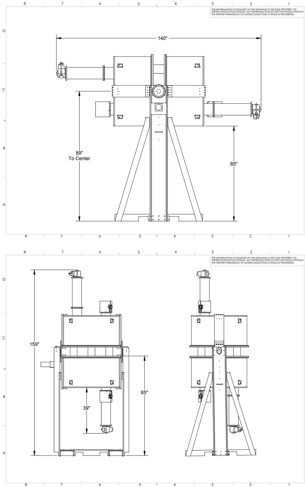
Figure 2: Schematic drawing of the magnet cryostat
